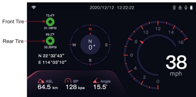
The green tire pressure icon means the connection is successful, and the gray means it is not connected.
